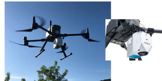
Figure 6: DJI M300 RTK y AA450
