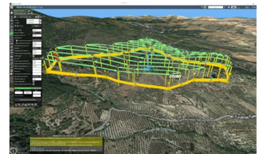
Figure 2: Scheduled flight plan with UgCS app with constant height on the ground from the IGN DTM.
